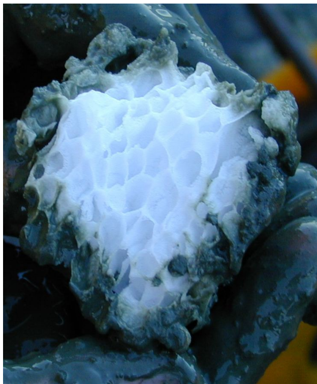
Figure 4. Structure of a gas hydrate (methane clathrate) block embedded in the sediment of hydrate ridge, off Oregon, USA. The gas hydrates have been found during a research cruise with the German research ship FS SONNE in the subduction zone off Oregon in a depth of about 1200 meters in the upper meter of the sediment – Image By Wusel00, via Wikimedia Commons
